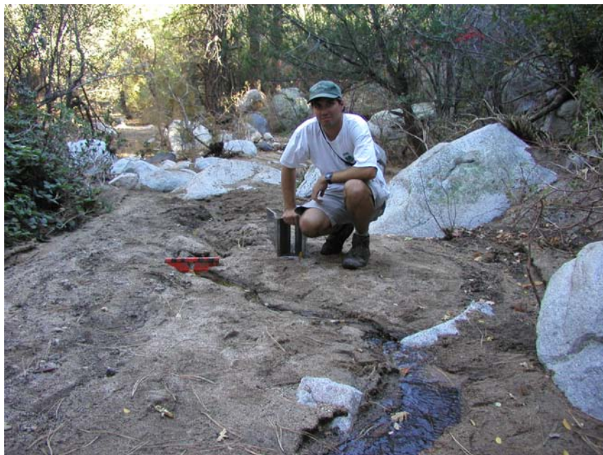
Fig. B2: The portable weir plate flow measurement procedure.
