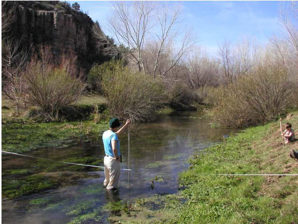
Fig. B3: The current meter flow measurement procedure.
