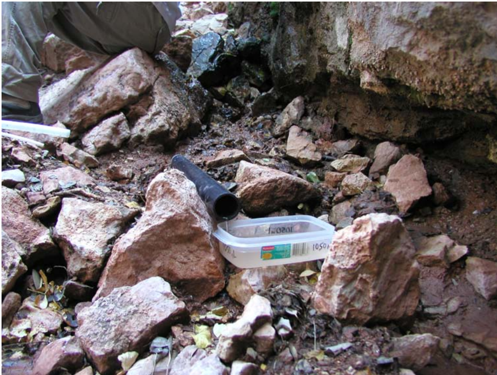
Fig. B5. The volumetric flow capture measurement procedure.
